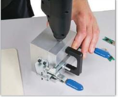
Securely close the mould shut with the component inside. Place the nozzle of the applicator into the injection hole in the side of the aluminium mould, and dispense the liquid resin, \_II the mould as quickly as possible and maintain trigger pressure for 5-15 seconds, after \_Iling to reduce shrinkage.
